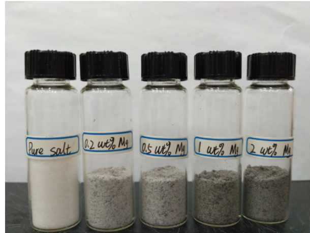
Fig. 5. Inorganic eutectic ternary carbonate salt with different composition of Mg [36].
