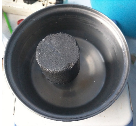
Fig. 10. EG impregnation with liquid PCM at 70°C.
