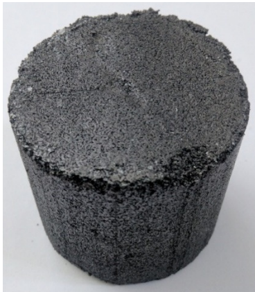
Fig. 9. Compacted EG porous foam.
